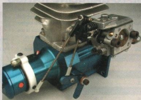
This Brison 3.2ci engine has a mechanical timing-advance ring coupled to its throttle arm. The ring advances and retards the engine timing as the throttle settings are changed.
