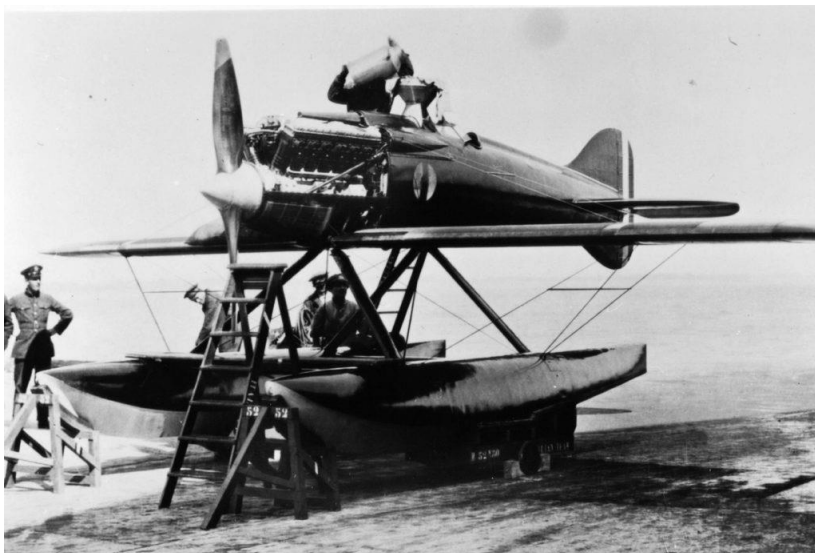
The home team brought four sleek Macchi M.52 racers to the 1927 competition in Venice, Italy, here showing off its 1,000 horsepower Fiat AS.3 DOHC V-12 engine. (San Diego Air and Space Museum Archive)
