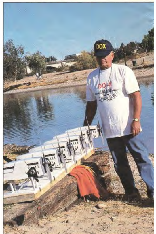
A clever design feature of the model Dornier is the engine module—a strong, removable section of the wing that supports all six engines along with their fuel systems, mufflers, servos and throttle radio. It's a completely self-contained unit that simply bolts to the wing, no other hookups required.
