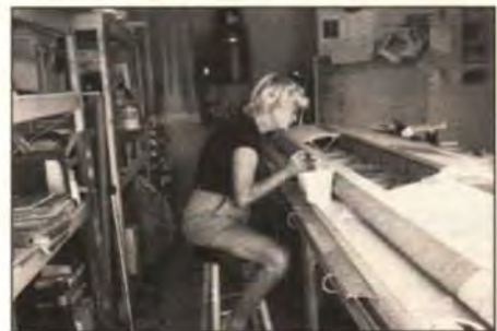
The tedious job of adding the corrugations to the wing leading edge was aptly handled by Carol Curtin, Bob's wife. Each of the 586 corrugations was done by gluing a piece of string to the leading edge—whew!
