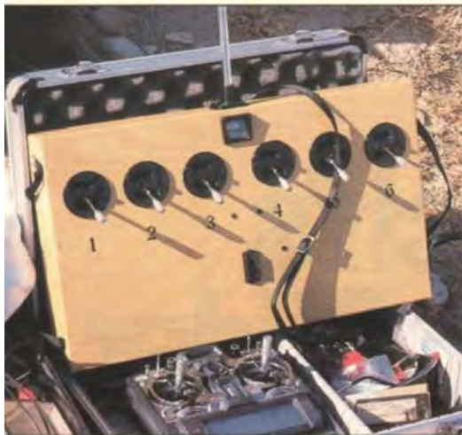
The Dornier uses a separate radio system to control the six engines; each engine can be controlled independently by the flight engineer by means of this special transmitter devised by John Wisniewski. John was the pilot for the flight, Bill Reed was the flight engineer.
