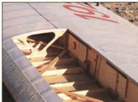
Close-up of the wing cavity where the engine module fits. Note the simulated sheet metal corrugations along the leading edge.
