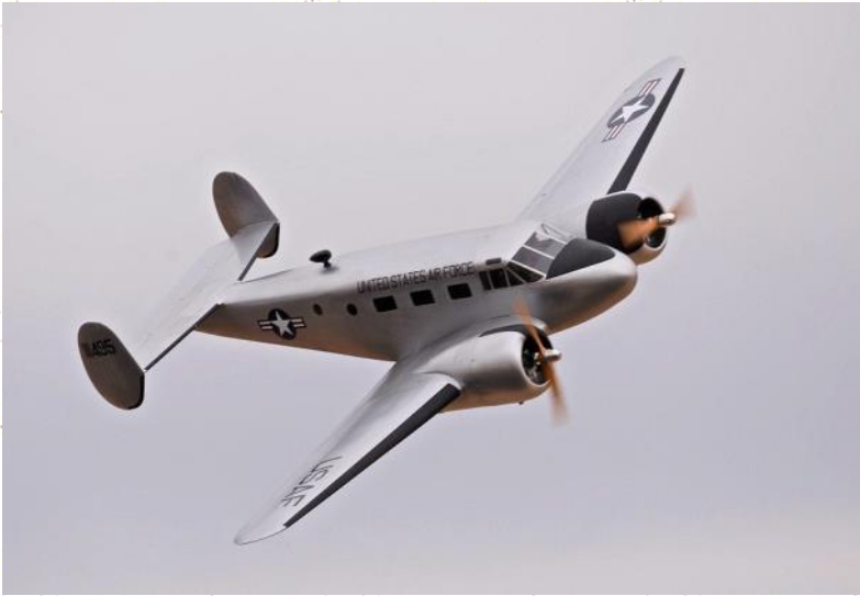
Larry Sheffield Beechcraft D18/C45 built from ZIROLI plans/parts. About 3 years in the making. Power by 2 DLE 35RA. It flies great!
