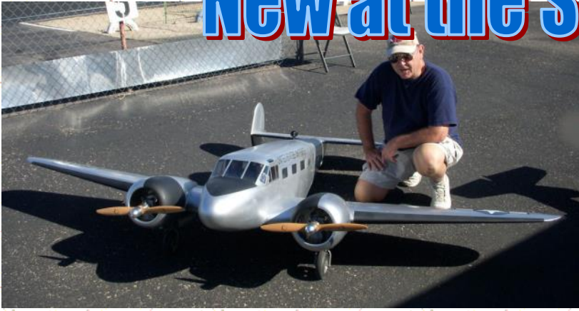
Larry Sheffield Beechcraft D18/C45 built from ZIROLI plans/parts. About 3 years in the making. Power by 2 DLE 35RA. It flies great!
